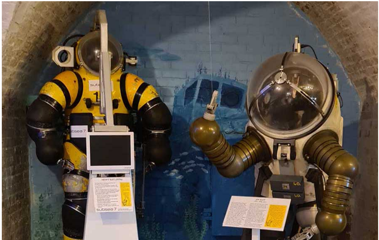
Newt and Jim suits: two one atmosphere diving suits. Credit: © Kevin Casey.
